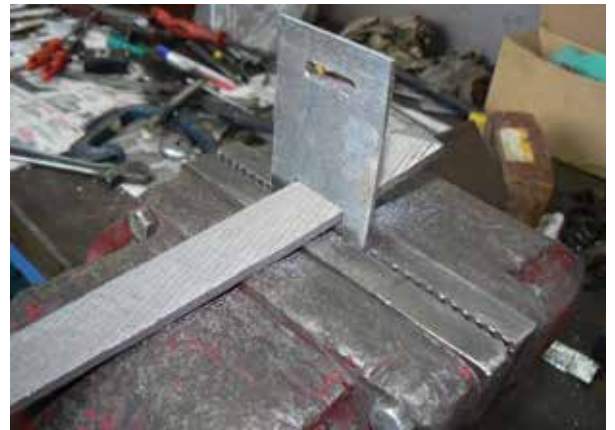
Fabricating a strap-type spring clamp.
