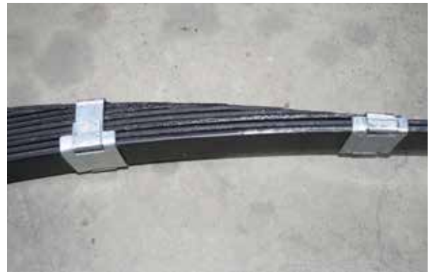
These flat strap clamps can be covered by the new spring gaiters.
