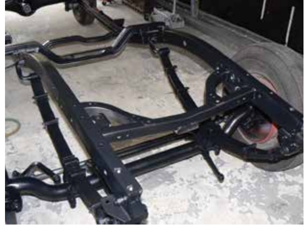
Note spring clamps on both sides of these front springs.
