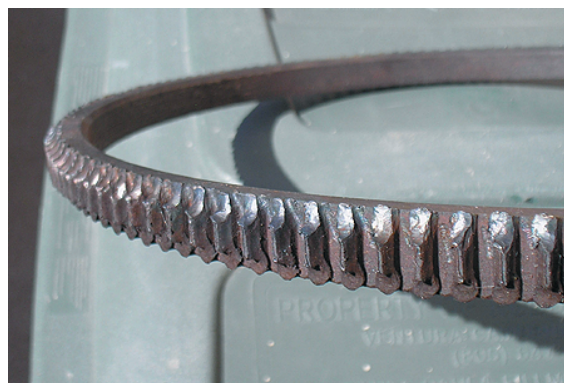
The flywheel ring was originally purchased with the car in 1976. Reversed and reapplied for the ACA Riverside National Meet. It had a hard life.
