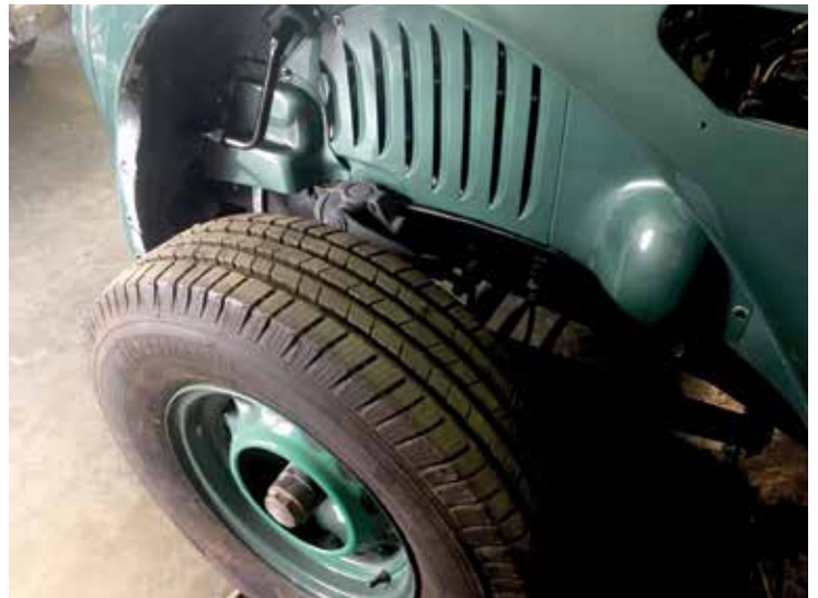
Horn tube, inspection panels, damper, and striped wheel detail.
