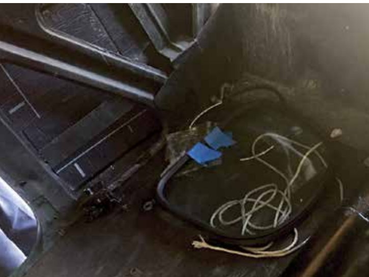
Cord-in-weatherstrip method: installing the back light glass.
