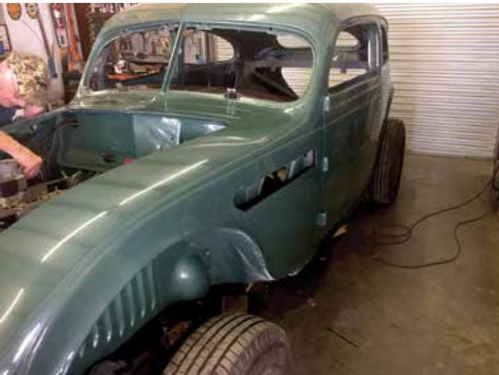
The body is back on the restored chassis. Reassembly begins! Here Phil works on wiring.
